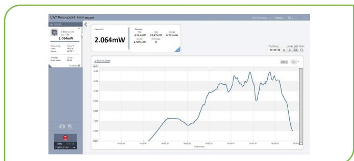
PMMManager™ is a powerful application software controlling and taking measurement data. It turns a PC into a laser power multi-channel analysis workstation. The PMMManager software features include extensive graphic display of data, advanced measurement processing, data logging for future review, printing of graphs and data, and the ability to connect additional devices during active measurements. Please see the PMMManager tutorial for more details on its capabilities.
